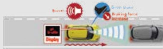
2. Deploys brake assist to increase braking force if the risk of collision is high and the driver panic brakes.
