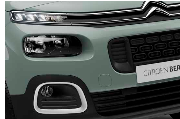
Front fog lights with cornering function
