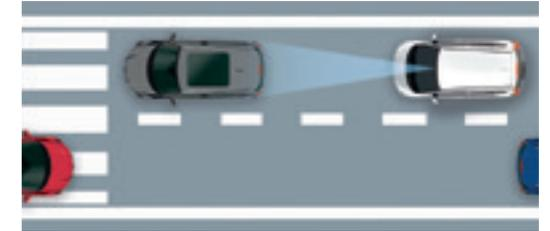
**1:** While driving around town between 3 and 20 mph, to give you the best chance of avoiding a collision, this system can monitor the distance between you and the car in front.
